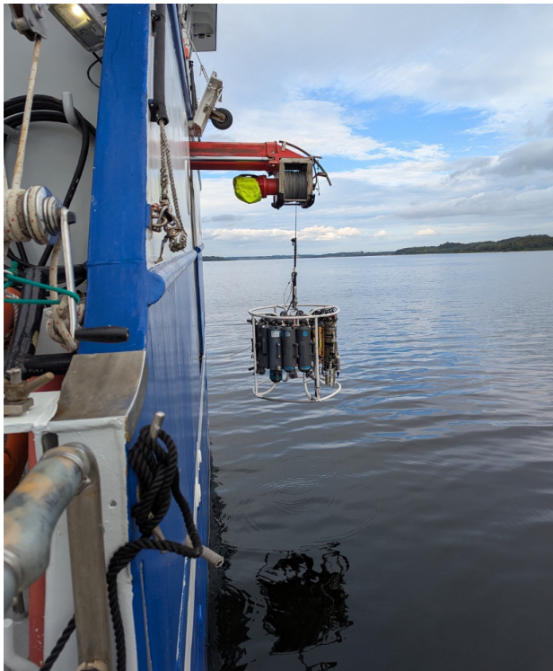
Photo: CTD cast during oceanographic expedition to collect water column samples from specific depths within the oxygen minimum zone. Copyright: Gonzalo Gomez-Saez
